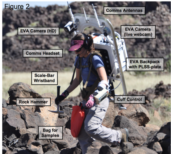
Fig. 2. A 2010 Desert RATS geologist crewmember traverses over a lava flow while on an EVA. Some of the tools available for EVA are shown here. The PLSS (portable life support system) plate is the large rectangular metal outline that allows the pack to fit into the suitports on the SEV, allowing for a safe and relatively quick ingress into the pressurized rover.
