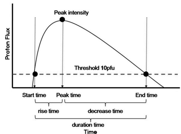
Fig. 1. Schematic diagram of a gradual SPE time profile.
