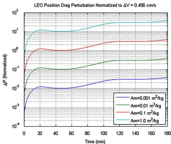
Fig. 2. Maneuver normalized atmospheric drag perturbations on a LEO object vs. time.
