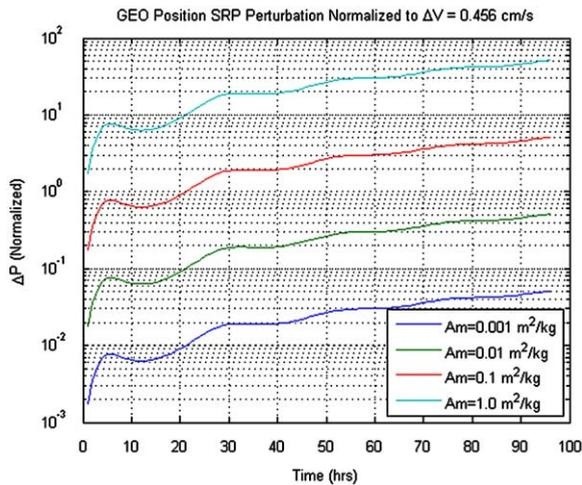
Fig. 1. Maneuver normalized solar radiation pressure perturbations on a GEO object vs. time.
