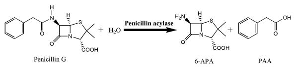
Fig. 1. Enzymatic hydrolysis of penicillin G.
