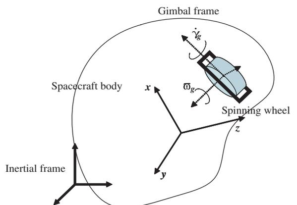
Fig. 1. Coordinate definition of spacecraft with one VSCMG.
