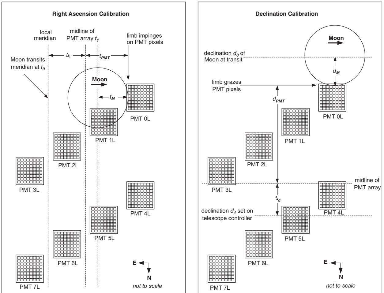
Fig. 1. Calibration of telescope position using PMT 0L. Each panel depicts the Moon moving through the eight PMTs in the left focal plane. The left panel shows calibration of right ascension ( $\alpha$ ) by measuring the time  $t_1$  that the right edge of the Moon impinges on the edge of the PMT 0L. The right panel shows calibration of declination ( $\delta$ ) by recording the telescope declination  $d_1$  for which the bottom edge of the Moon impinges on the top edge of PMT 0L.
