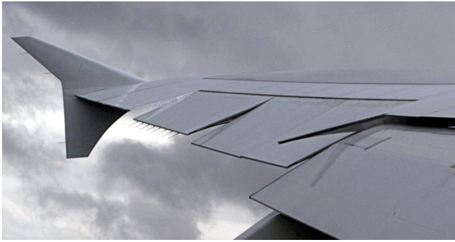
Fig. 1. Airbus A380 wing with multiple control surfaces deflected showing the large gaps created [3].
