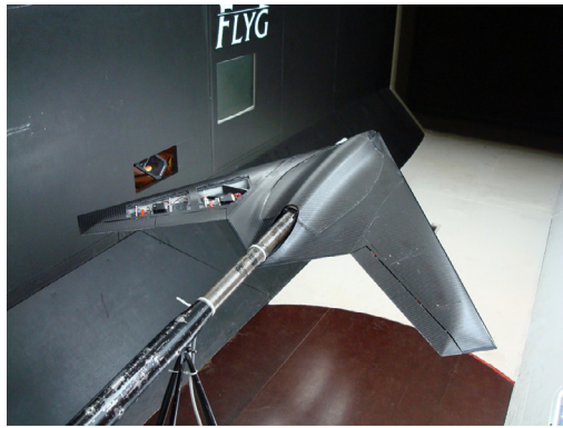
(a) The Swing model in the low-speed wind tunnel.
