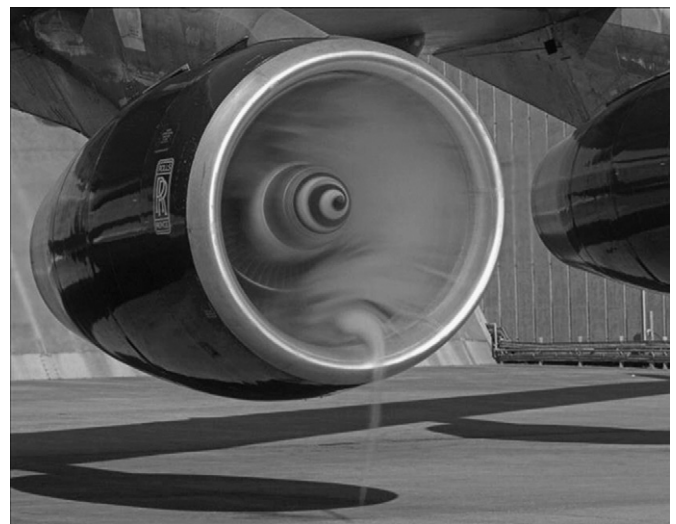
Fig. 1. Ground vortex ingestion on a RB211-524G in static aircraft conditions (photograph by Peter Thomas).
