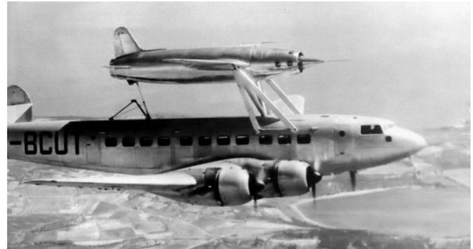
Fig. 1. The experimental ramjet aircraft Leduc 0.10 [5].
