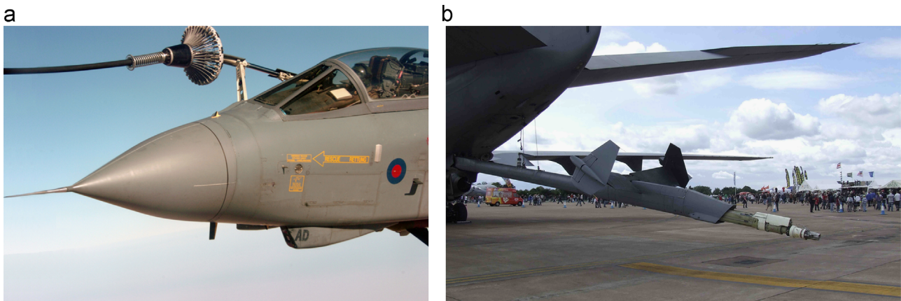
Fig. 1. Refuelling methods. (a) Hose and drogue. Photo by US Navy, (b) Flying boom. Photo by P.R. Thomas.
