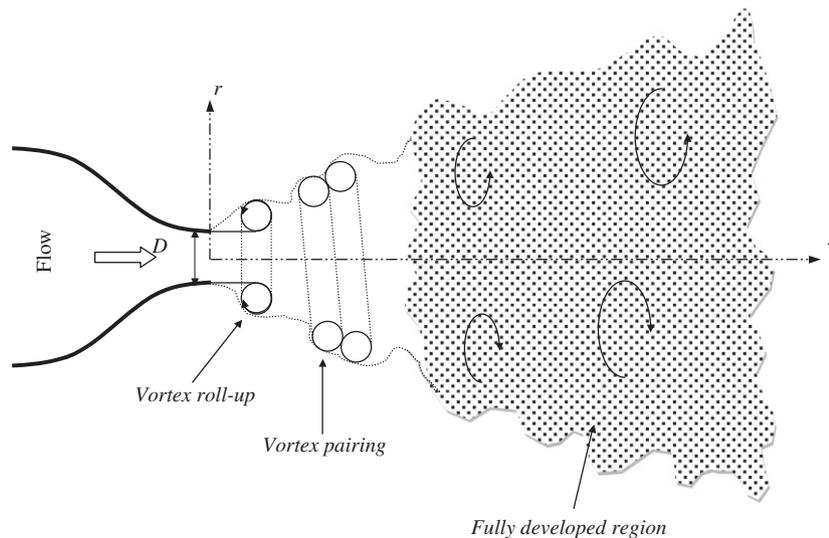
**Fig. 2.** Flow features of the free round jet.
