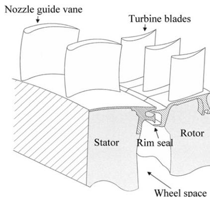
**Figure 1** Typical high-pressure turbine stage showing rim seal and wheel-space.
