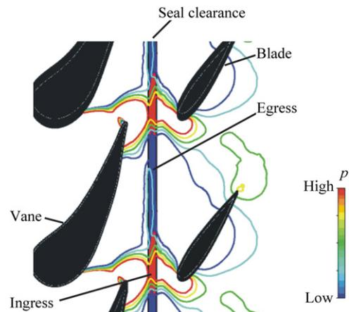
**Figure 2** Computed pressure contours between vanes and blades of experimental rig (adapted from Zhou et al. [1]).
