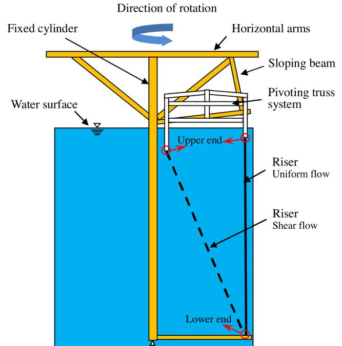
**Fig. 1.** Sketch of experimental arrangement.
