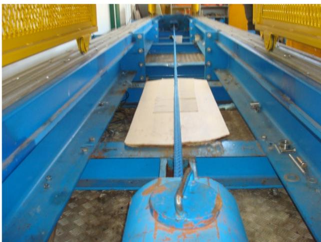
Fig. 1. Braided rope on tensile test frame before test.
