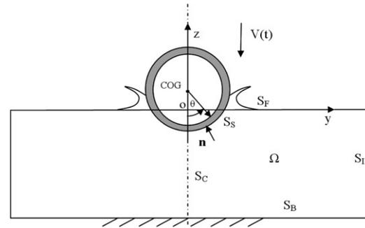
Fig. 1. Coordinate system and definitions.
