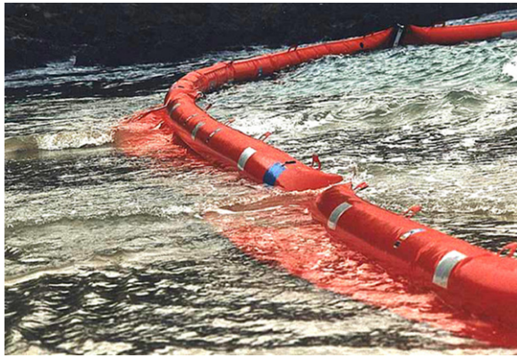
Fig. 1. Boom behaviour under a strong current.
