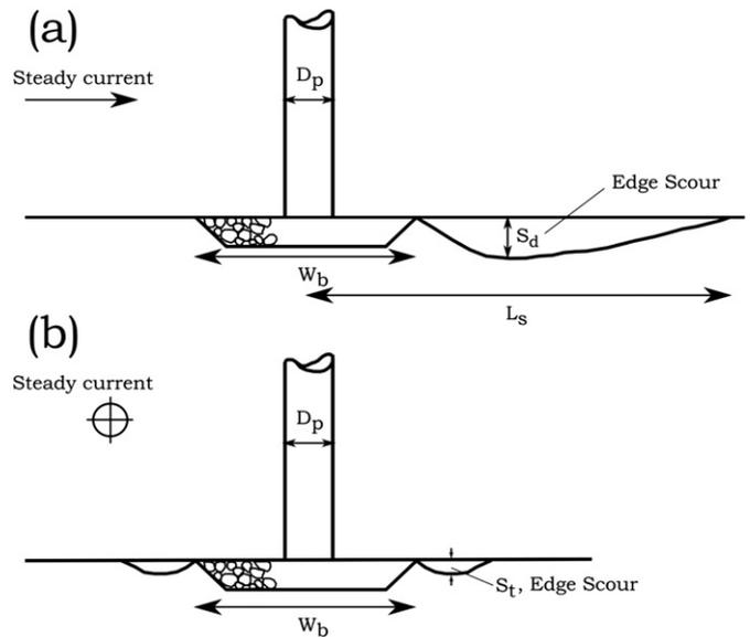
Fig. 2. Definition sketch (schematic) for the setups with scour protection installed flush with the sea bed. (a) scour hole generated by current downstream of scour protection; (b) scour generated by current at the transverse section of the scour protection. Note that the setup for the scour test in combined waves and current are identical, and the current and waves are collinear.
