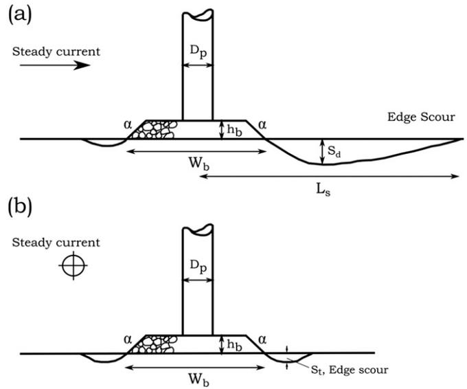
Fig. 1. Definition sketch (schematic) for the setups with scour protection installed on the sea bed. (a) scour hole generated by current downstream of scour protection; (b) scour generated by current at the transverse section of the scour protection. Note that the setup for the scour test in combined waves and current are identical, and the current and waves are collinear.
