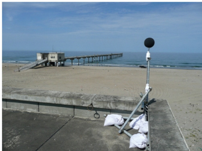
Picture 1. Location of the sound meter near HORS.
