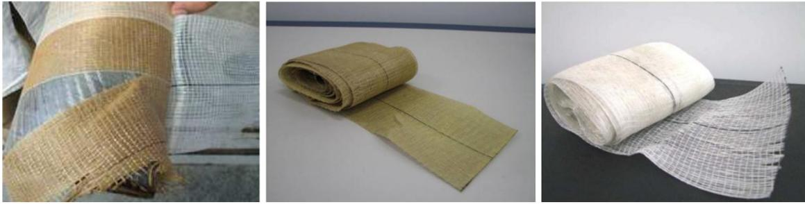
Fig. 1. High strength tapes used in flexible pipes. Middle: Kevlar. Right: PET.
