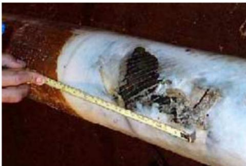
Fig. 3. Damaged tape in flexible pipe.
