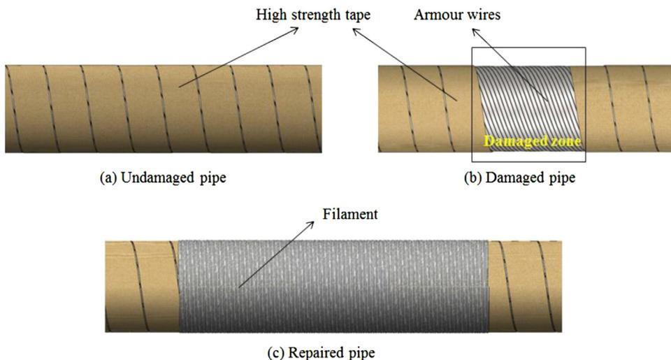
Fig. 4. Schematic diagram of damaged and repaired pipe.
