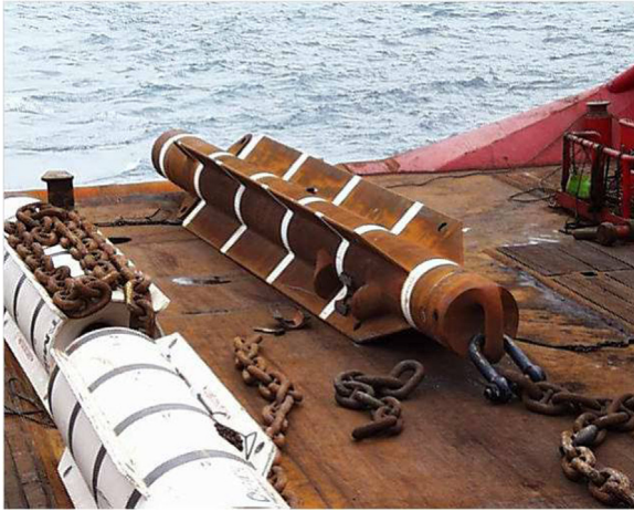
Fig. 1. Torpedo type offshore anchors and chains used by Petrobras (Petrobras archive).
