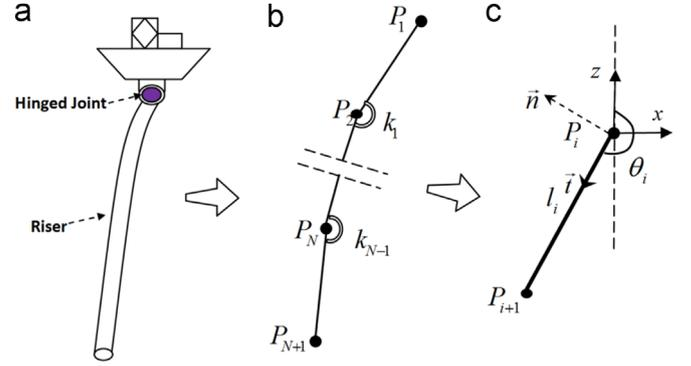
**Fig. 2.** Physical model of a freely-hanging marine riser: (a) a riser in reentry, (b) its dynamic model, and (c) magnified  $P_i$  node.
