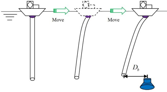
**Fig. 1.** Reentry process of a freely-hanging riser.  $D_b$  is the lateral distance between the riser lower end and the seabed wellhead, uncertain for the oscillation after movement.
