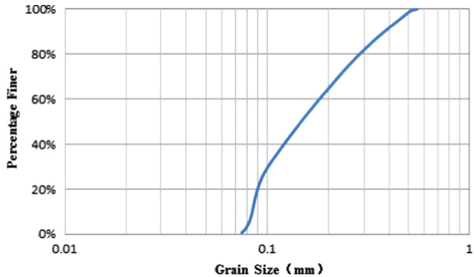
Fig. 2. Grain size distribution curve of sandy deposit.
