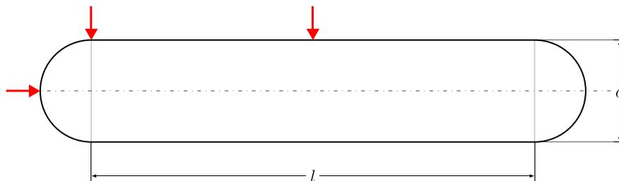
Fig. 2. Cylindrical hull with hemispherical end closures showing axial, end transverse and centre transverse excitation of the cylinder.
