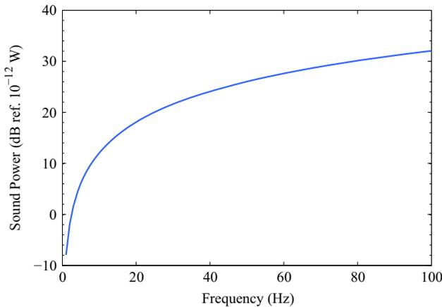
Fig. 1. Radiated sound power from a dipole with 1 N amplitude.
