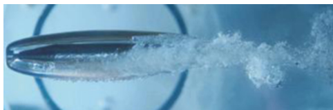
Fig. 1. Water tunnel experiment on supercavitation.
