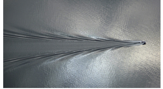
Fig. 3. Photograph of a fast planing motor-boat exhibiting a narrow wake (source: http://en.wikipedia.org/wiki/Wake ).
