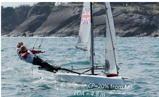
Fig. 3. Photograph of the Aura in full scale with a forwards crew position.
