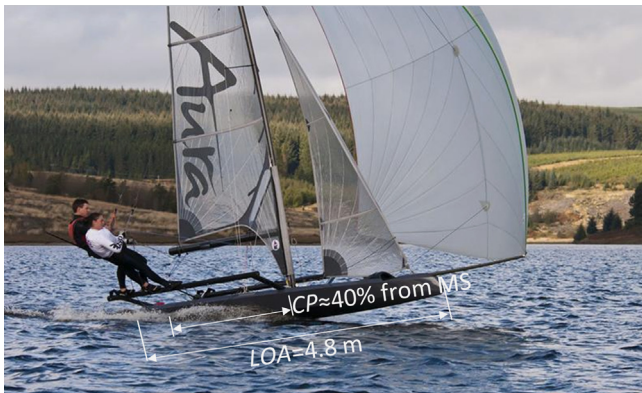
Fig. 2. Photograph of the Aura in full scale with an aft crew position.
