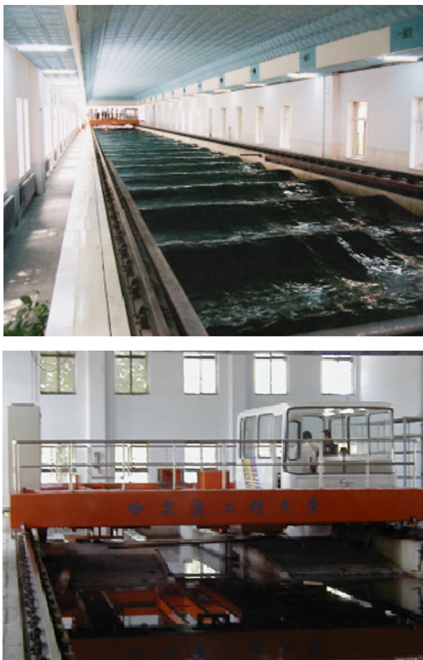
Fig. 1. Towing tank and towing carriage.
