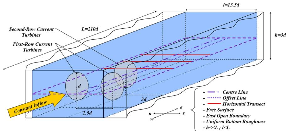
**Fig. 1.** Idealized channel, multi-disc case – this conceptual diagram represents the multi-disc test geometry and dimensions as well as the locations where horizontal transects (red solid lines), centre and offset lines (purple solid and dotted lines) have been taken. (For interpretation of the references to color in this figure legend, the reader is referred to the web version of this article.)
