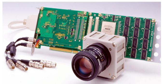
Fig. 3. High-speed camera and image grabber.
