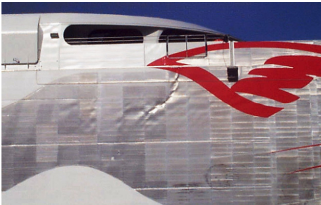
Fig. 2. Side shell buckling as a consequence of severe slamming loads, Hull 50 of Incat Tasmania.
