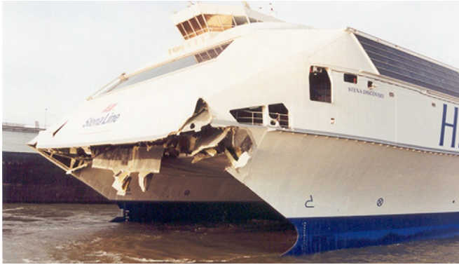
Fig. 1. Damage of bow structure on HSS 1500 Stena due to severe slamming loads.
