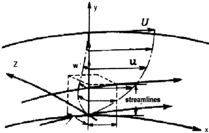
Fig. 1. Typical velocity distribution in a 3D boundary layer with a secondary flow along the z-axis.
