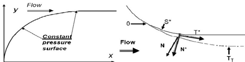
Fig. 2. Flow scheme (in the left) and comparison of its boundaries iteratively changed during solving of the boundary-value problem (1)–(3) (in the right).
