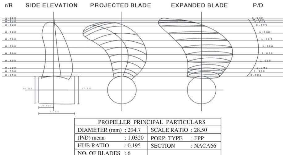
Fig. 3. The geometry of propeller model.
