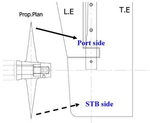
Fig. 1. Variation of rudder incident flow caused by propeller wake (port side view).
