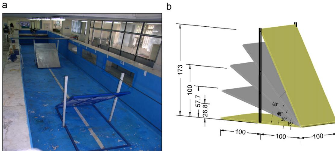
Fig. 1. An overview of two inclined beds installed in the laboratory water tank and the changeable slope angle.
