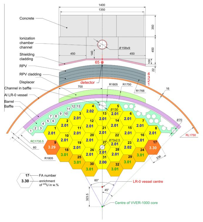
Fig. 1. Section of the mock-up in the x-y plane (Dimensions in mm). Basic configuration.
