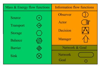
Fig. 1. Symbols of Multilevel Flow Model.
