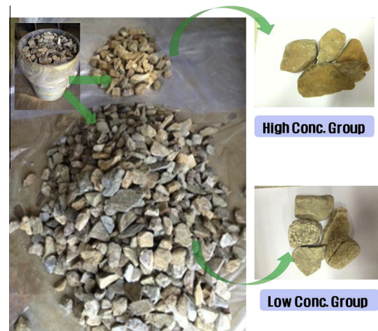
Fig. 1. Gravel contaminated with uranium.
