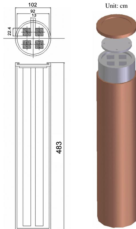
Fig. 1. Schematic illustration of a KDC-1 canister.
