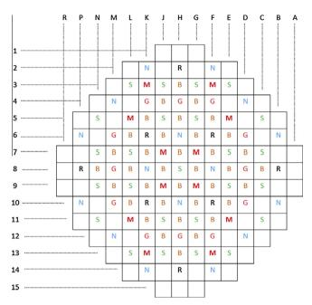
Fig. 1. Representative control element pattern in a PWR transmutation core.
