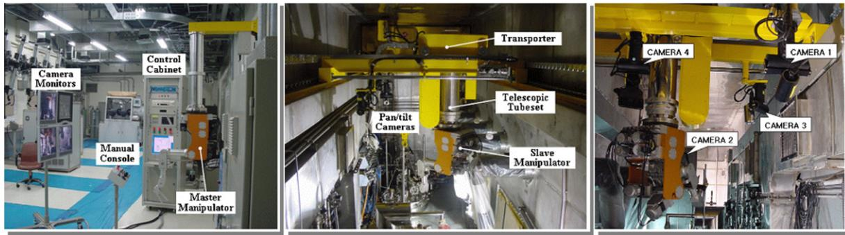
Fig. 1. Master manipulator (left), slave manipulator (center), and cameras (right) in the ACPF.
