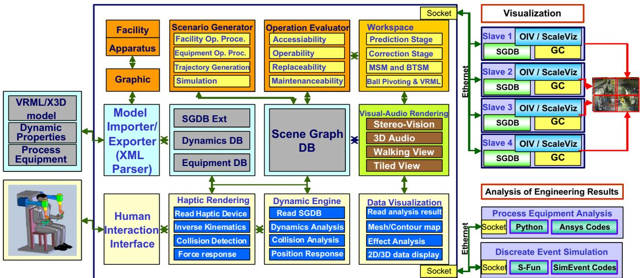
Fig. 2. Schematic diagram of the system architecture for a modeling and simulation tool.
