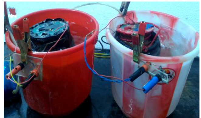
Fig. 1. Photograph of working dual chambered MFCs treating urine as a substrate in anodic chamber.
