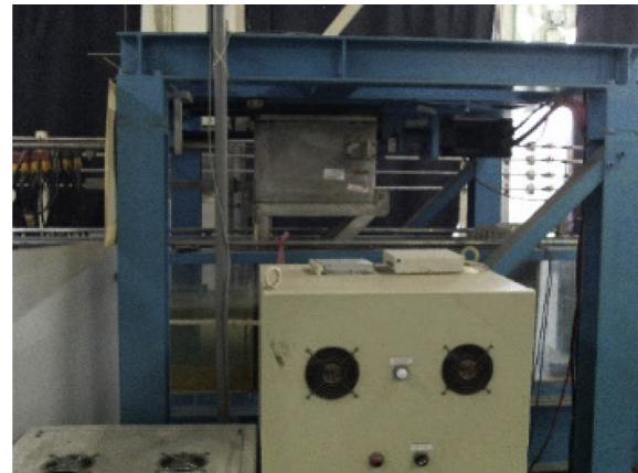
Fig. 2. Wave generator installed at the end of open channel shown in Fig. 1.
