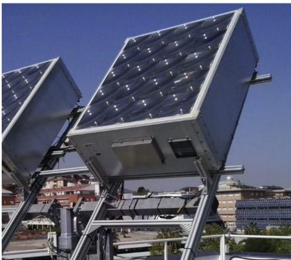
Fig. 1. Left: photograph of the HCPV module considered in this study. Right: scheme of the experimental set-up to measure the I–V characteristics of the HCPV module and the main atmospheric parameters.
