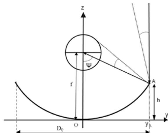
Fig. 1. Rim angle of the solar parabolic concentrator.
