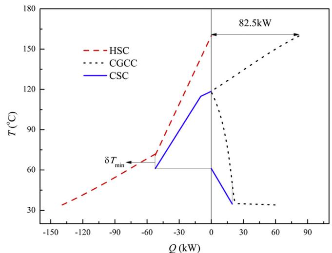
Fig. 2. The cycle with rectification heat recovery by total strong solution.
