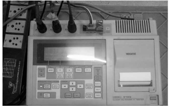
Fig. 4. Hioki 3165 make power analyser used for conducting power study.
