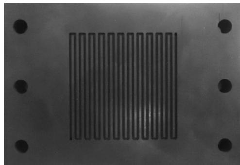
Fig. 3. Anode flow field machined on graphite plate.
