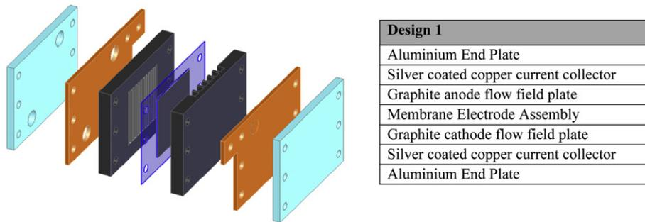
Fig. 2. Exploded view of air-breathing fuel cell.
