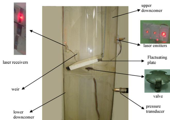
Fig. 1. The rig and its components.
