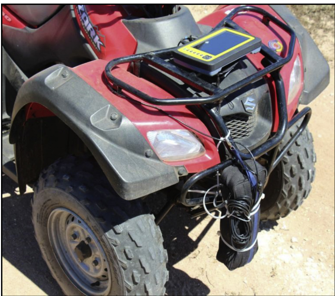
Fig. 1. Photographs of the measuring system that was utilised during the in situ measurements. The photographs show the casing with the detector mounted to the frame and the tablet with an inbuilt GPS on the carrier.
