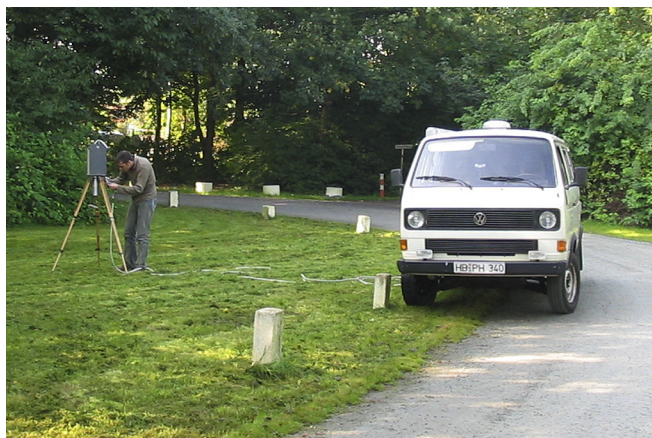
Fig. 2. Exemplary setup for the recording of an in situ gamma spectrum. The hpGe detector is mounted on a tripod facing downwards. The associated electronics remain in the transport van.
